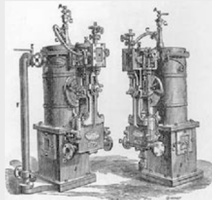
Diagram (1883) of Chaplin's patent seawater distilling apparatus, as used for sailing vessels, with steam pump attached for circulating water.
