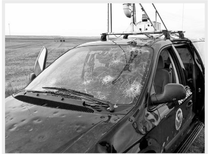
A NOAA vehicle shows damage from multiple large hailstone impacts.
