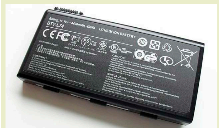
A typical lithium-ion battery from a laptop computer.
