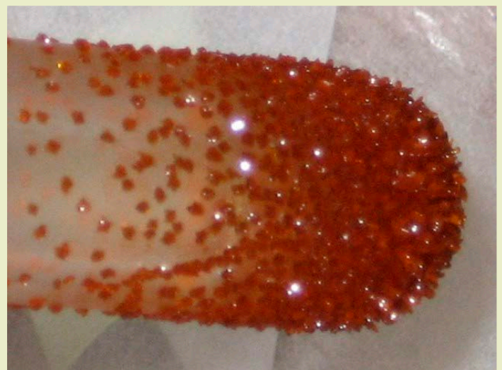
Ferrocene crystals deposited on a rod after purification by sublimation.
