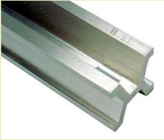
Closeup of National Prototype Meter Bar No. 27, made in 1889 by the BIPM and given to the United States, which served as the standard for defining all units of length in the United States from 1893 to 1960. With concerns about the effects of temperature and age on the bars, in 1960, the SI changed the standard of length to define the meter by the wavelength of light of a spectral line of krypton-86. Today, the meter is more precisely tied to the speed of light, a universal physical constant.
