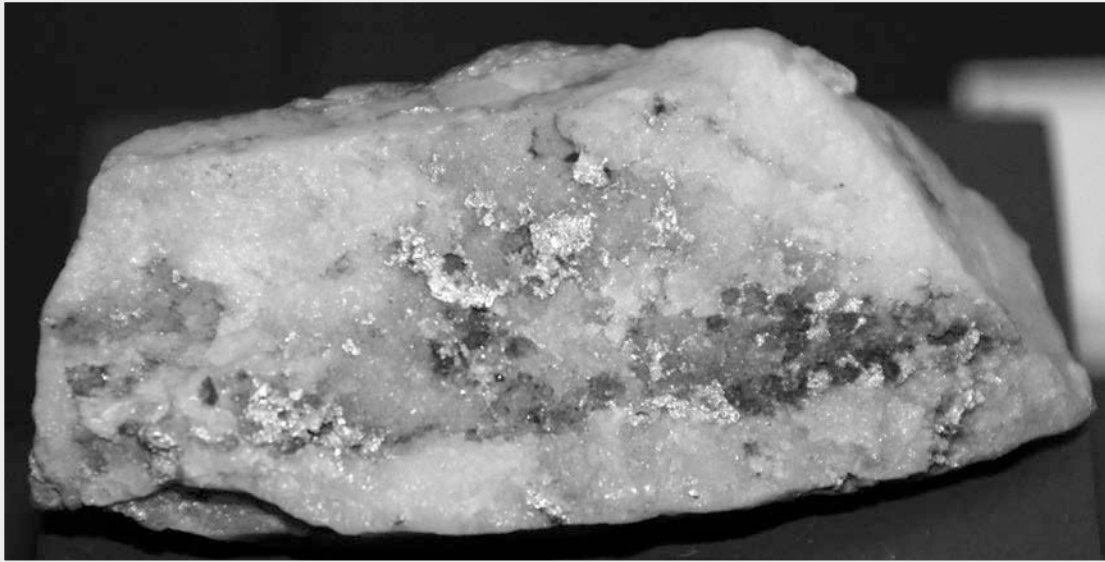
A sample of gold-quartz hydrothermal vein from the Maryland Mine at Potomac, Maryland, USA.
